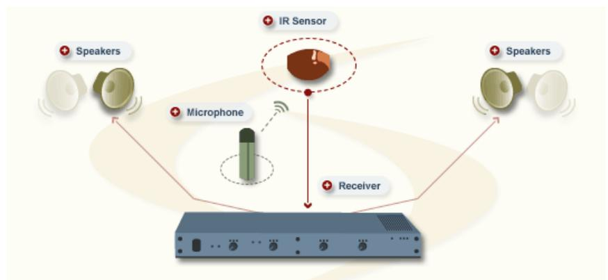
Infrared classroom audio has emerged as the perfect technology for delivering clear instruction to all students, mitigating poor acoustics and high ambient noise levels.
